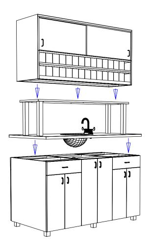
The 946-60 color bar ships in 5 pieces (3 base cabinets, 1 riser/counter assembly and 1 upper cabinet.)
